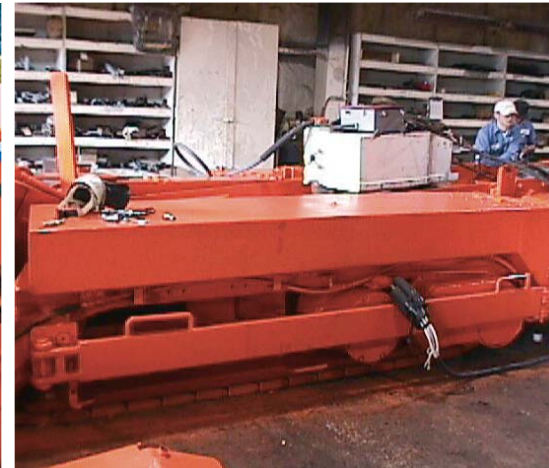
Englo Type 18 Being Retrofitted on a Joy 14cm15 Continuous Miner
